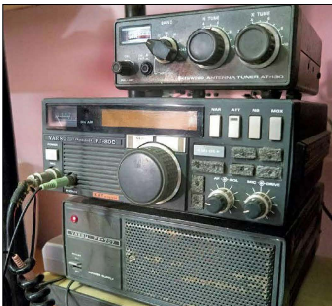
New radio equipment and parts for repairs can be hard to come by in Cuba. CO2YQ has repaired his Yaesu FT-80C with custom cut replacement buttons made from foam.
